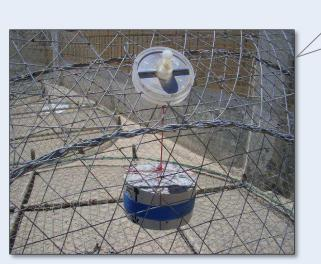
The study, prepared by the Kuwait Institute for Scientific Research, suggested a solution to the problem of ghost fishing, where an automatic system was designed to open the fish trap.
