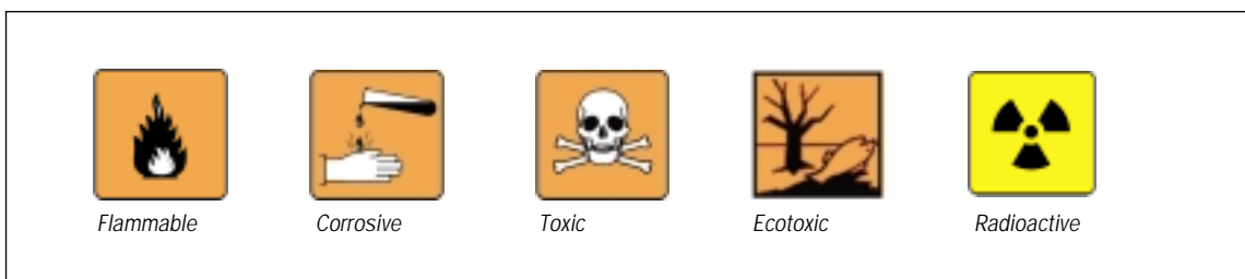
Figure 2: Examples of hazardous properties
