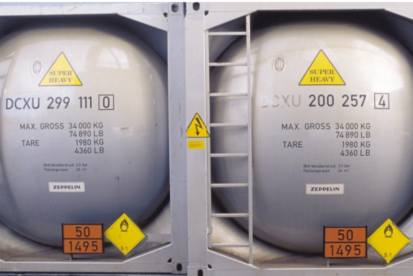
Tanks of chemicals for shipping by boat labelled with signs. A numeric code indicates the contents. Espen Bratlie / Samfoto
