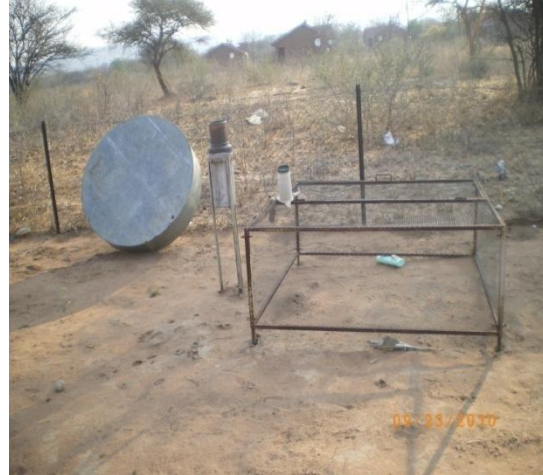
Fig 1 (b) showing a dysfunctional evaporation pan (Source: Fieldwork)
