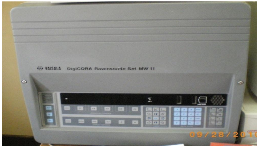
Fig 3 Showing a Digicora at SSKA, reported to have not worked since October 2009.
